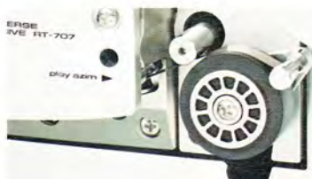
PAUSE MODE: The pinch roller stays close to the capstan, while tape is in contact with heads. Start-up is instant.
