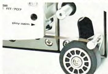
STOP/FAST FORWARD/REWIND MODE: The pinch roller is far away from tape path, to enable easy tape loading and smooth tape transport.
